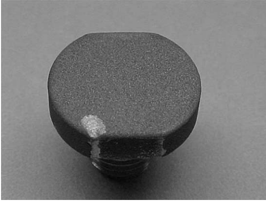
Fig. 8. LN specimen with metallic glass coating that has partially failed near the near edge.
